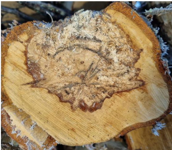
Birch with light, loose rot. The entire rot surface, including the black ring, is counted as rot damaged.
