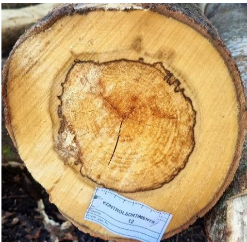
Tick rot in aspen – the entire surface inside the thin, dark ring (including the ring) is assessed to be loose/dark rot. The pale grey or light brown surface outside the ring is not counted as rot.
