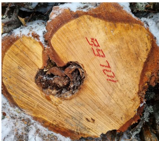
Birch with dark, loose rot. The entire rot surface is counted as rot damaged.
