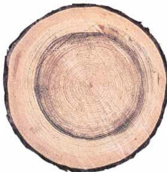
Disc with ring-shaped dark, solid rot. The rot inside the ring has a colour shade that is on the limit of what can be accepted as 'light' rot. Only the area of the ring is counted as rot damaged.
