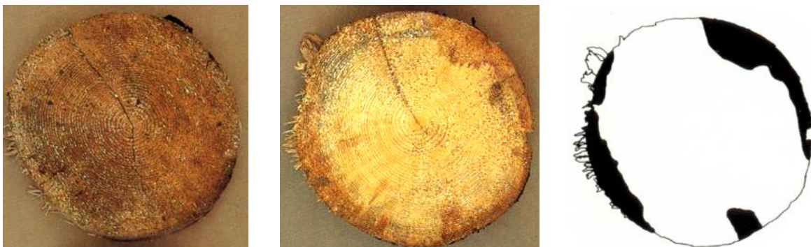
Figure 6. Storage decay in spruce. Left: end surface of the log; Middle: a cross-section 15 cm from the log end; Right: Storage decay highlighted in black. Log diameter 20 cm, 25% storage rot (Rötskador i massaved, Swedish Forest Agency, 1989).
