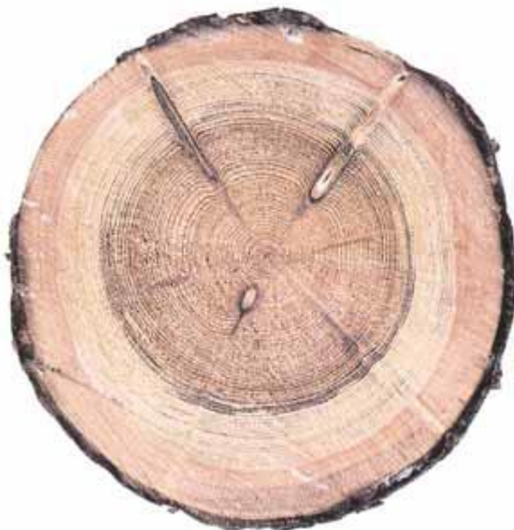
Disc with moderate brown forest rot. The rot is assessed as dark rot. The entire dark area is counted as rot damaged.
