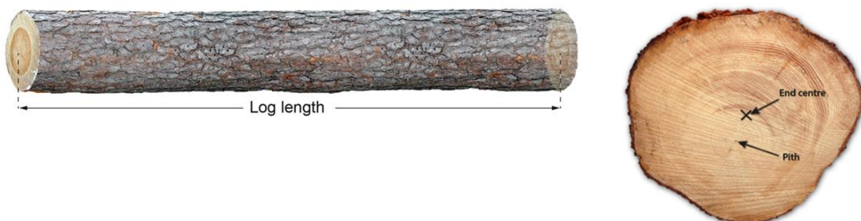
Figure 2. Log length is the shortest distance between the centres of each end of the log. The centre is the geometric centre of the end surface.
