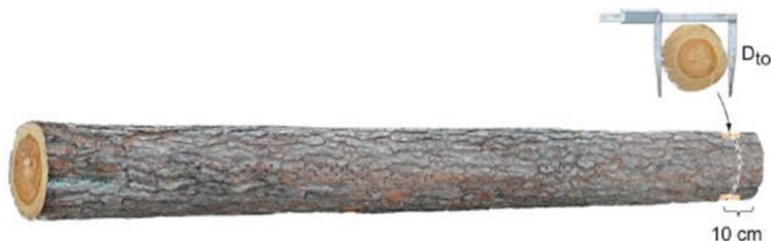
Figure 10. Measurement point for diameter in top measurement.
